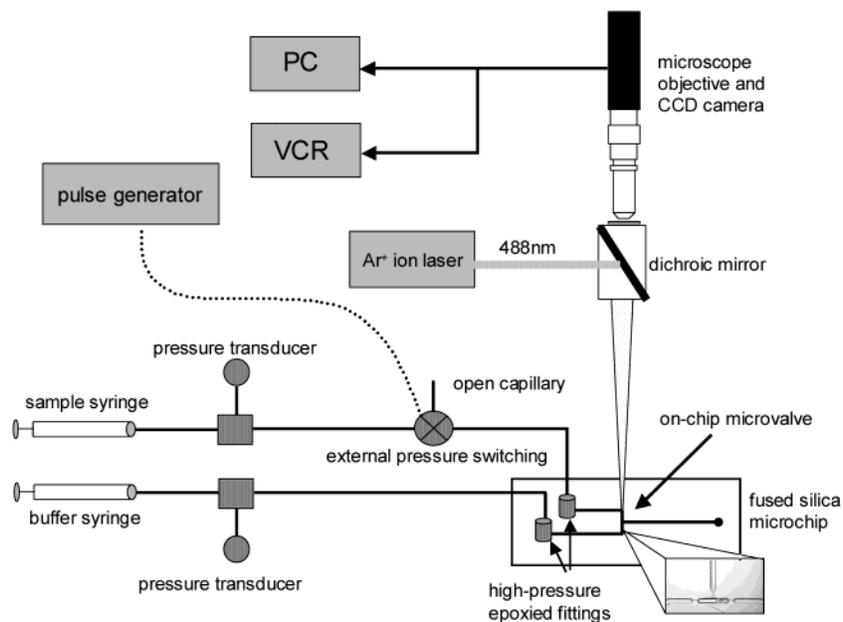
Figure 2. Schematic of the injection quantification apparatus.
