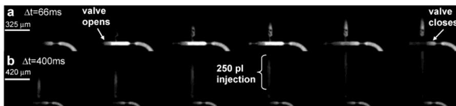
Figure 4. Time series of a 250 pL injection. Series a shows the opening and closing of the injection valve. While the motion of the polymer element cannot be seen directly, the presence of fluorescence in the injection region is indicative of valve actuation. Series b displays the movement of the sample plug into the injection channel.
