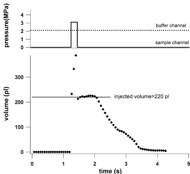
Figure 5. Volume of sample fluid present in the valve region and injection channel during an injection cycle, indicated with diamond markers. The volume of sample fluid is calculated from the fluorescence, as shown in Figure 3. The injection volume is 220 pL. The buffer channel (dashed line) is held at constant pressure, 2.1 MPa (300 psi). The sample channel (solid line) is pressurized to 3.1 MPa (450 psi) at 1.20 s and depressurized at 1.46 s.
