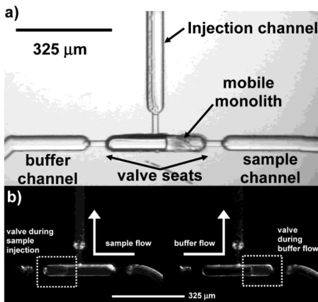
Figure 1. (a) Micrograph of the injection valve. In the position shown, fluid from the buffer input at left travels down the injection channel at top. Sample fluid at right is isolated from the rest of the system. (b) Movement of the polymer element (mobile monolith) allows control of the fluidic pathways.
