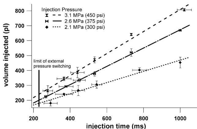
Figure 7. Injected volume as a function of injection time and pressure. The buffer channel pressure is held constant at 1.0 MPa (150 psi) below the injection pressure. Error bars indicate the standard deviation of the injection volume and duration.
