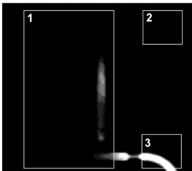
Figure 3. Micrograph of the injection valve with the integration areas highlighted. The integrated signal from region 1 is due to the flow of dye solution into the injection channel and is used to calculate the injected volume. Signal measured in region 2 is used to determine background fluorescence. Region 3 comprises a known volume of sample, allowing calibration of fluorescence intensity to volume of solution injected.
