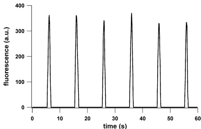
Figure 6. Fluorescence intensity measured downstream from the valve. Injections are performed at 0.1 Hz, with a 500 ms duration. The buffer channel is held at constant pressure, 2.1 MPa (300 psi); the sample channel is pressurized to 3.1 MPa (450 psi) during injection.
